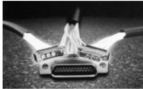
Size Comparison: Above; Nano, Below; Micro-D
